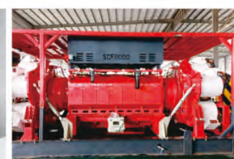
8000HP连续满载全电动压裂装置 8000HP Continuous Full-Load Fully-Electric Fracturing Unit
