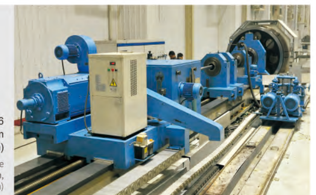
深孔钻镗床 DDBI 60×60/16 (钻镗孔最大长度6000mm 镗孔最大直径φ600mm 钻孔最大直径φ110mm) Deep Hole Drilling & Boring Machine (Max.Length 6000mm, Max.Boring Dia. φ600mm, Max.Drilling Dia. φ110mm)
