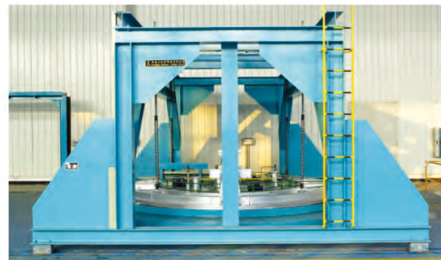
气体淬火炉 \phi 4000 \times H2000 Gas Carburizing Furnace
