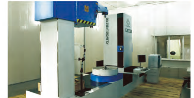
齿轮测量中心P300 \phi 3000 Gear Measuring Center
