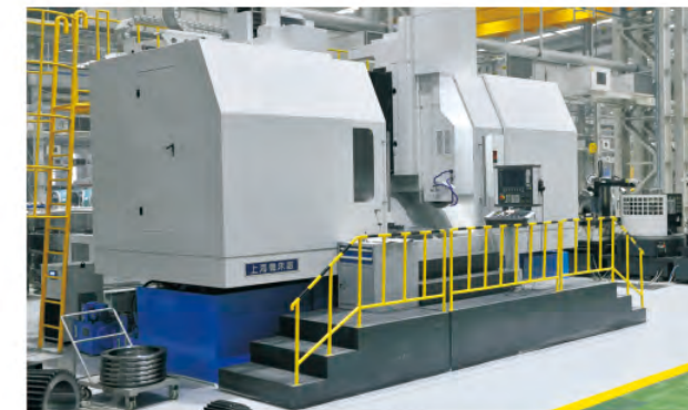
数控立式复合磨床H322 (最大磨削外径φ1600mm) Vertical NC Combined Grinding Machine (Max.O.D. φ1600mm)
