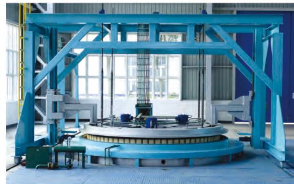
MDR991井式加热回火炉 \phi 4000 \times H3000 Well-type Tempering Furnace MDR991
